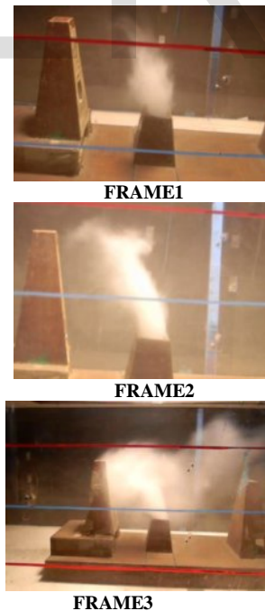
Fig7. Plume trajectory at k=0.5 with 4x2 cross-section throughout the mast with 45 degree opening and 9cm above
